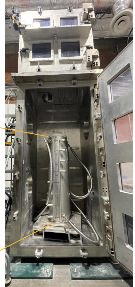
Test Sample 1 m column of uniform water ice distribution
